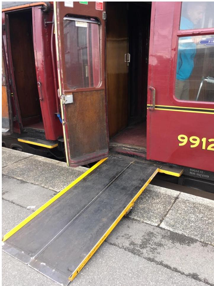
Figure 1 - Mobility access ramp in use on one of our 1950's carriages
